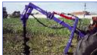
Planetary drive posthole diggers with hydraulic down pressure, various auger sizes.
