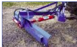
6' medium heavy duty hydraulic grader blade. Hydraulic angel and tilt plus manual offset.
